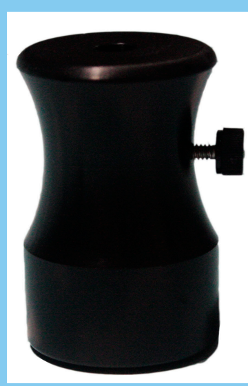
Probe: MP- RP90 Spot size ~ 2mm. Works in wide spectral range
