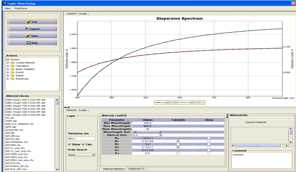
Fig. 16 Optical constants of conductive polymer determined from the measurement.
