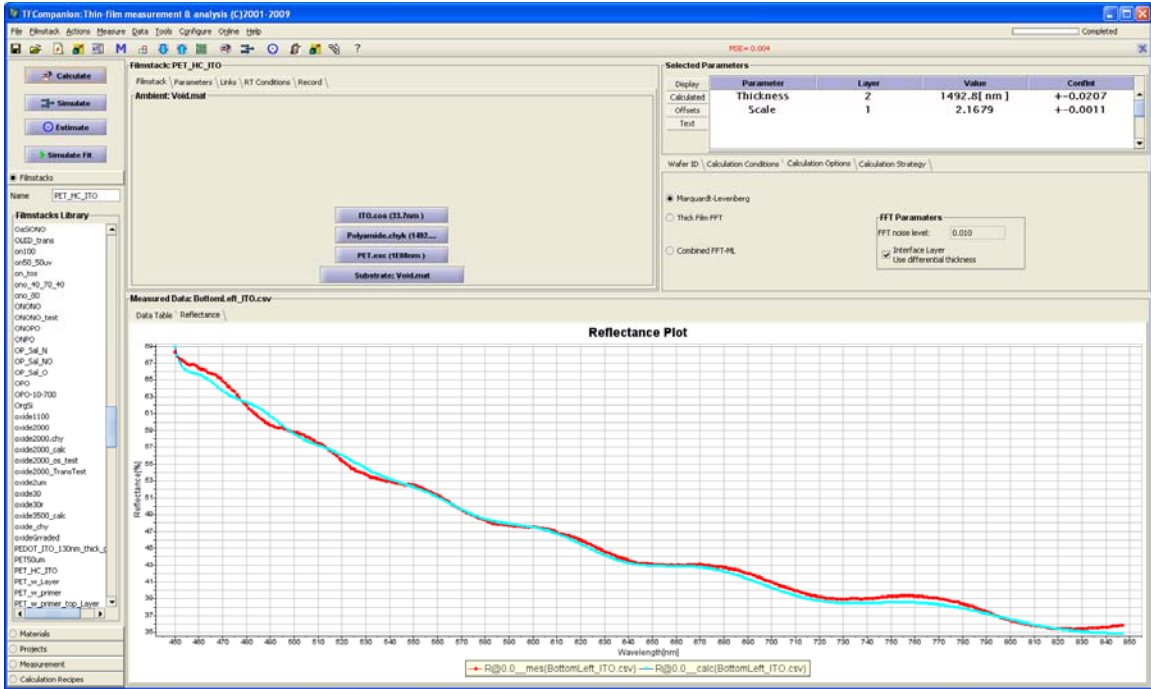
Fig. 3. Fit of the model to measured data. Both ITO and HC layers thickness is determined. Model data now follows the fringes and the fit is much better as compared to the Fig. 2 where HC layer was ignored.
